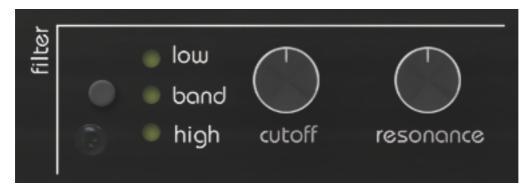
The SID chips are equipped with a multimode resonant filter. The filter is the analog section of the circuit and its warm/dirty sound contributes to the authentic SID character.
